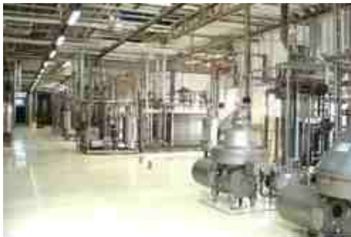
Smooth flooring with no cracks or holes is easy to clean
