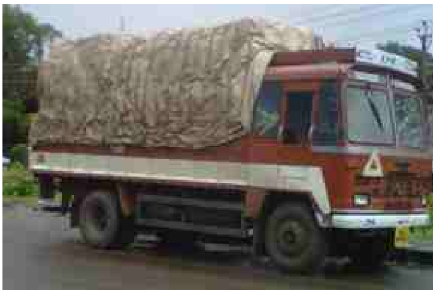
Cover the road vehicles with tarpaulin sheet to protect against rain and birds, insects.
